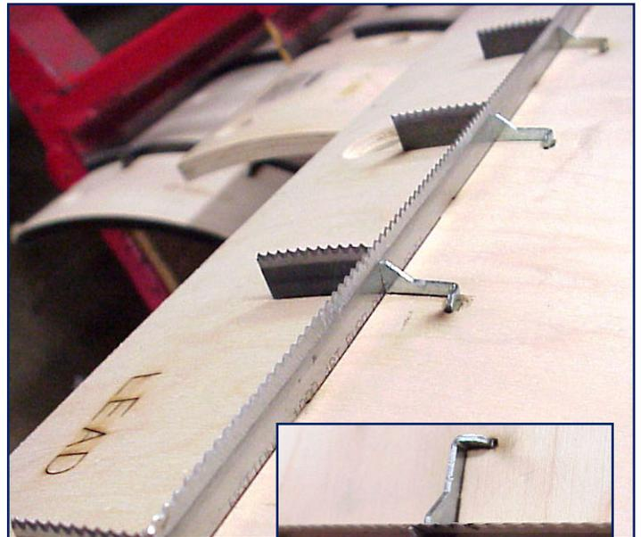
*LeGards are positioned opposite the lead edge trim knives and include a bent "tail" which anchors it in position.*
