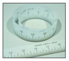
Stretch Measuring Tape is used for laying out of rotary die boards. Compensates for differences between flat and rotary measures. Available for 1/2" and 5/8" wood for a 66" cylinder, .970 high rule.
