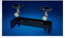
**Heavy Duty Hydra Jacks** Heavy Duty Hydra Jacks are best suited for label presses greater than 16," as well as carton presses 13" and up.
