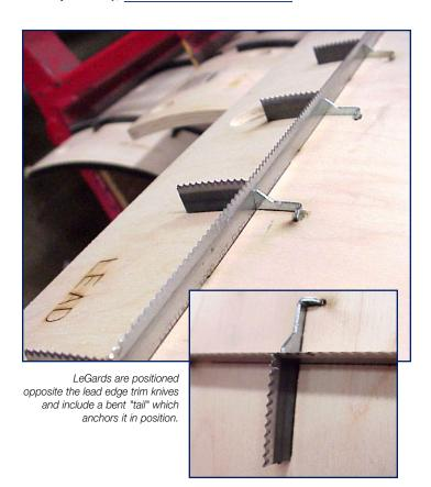
**LeGards** can also be used in other situations, such as tight miter tangent areas, which are prone to opening during diecutting. These areas previously required welding in order to hold them together, LeGards offer an easy and effective solution.
